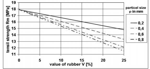
Fig. 2. Influence contents of rubber powder V[%] and sizes of grains( $\varphi = 0.2$ ; 0.4; 0.6 and 0.8 mm) on endurance on extension Rm [MPa] – for pressing
