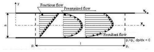
Fig. 2.4. Velocity distribution in the flat aperture at pressure difference and upper plate moving according to the direction of pressurized flow
