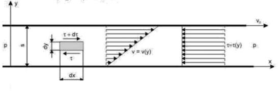
Fig.1. Flow in the flat aperture caused by the motion of upperplate
