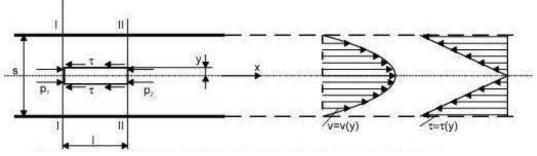
Fig. 2.3. Scheme of flow in the flat aperture caused by the pressure difference
