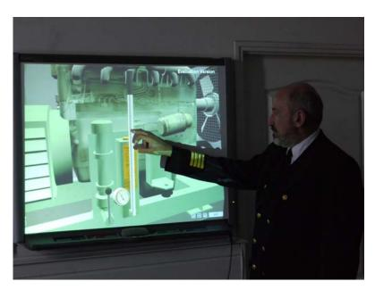
$Fig.\ 6\ LER3D\ Engine\ Room\ Simulator-Application\ of\ touch\ screen\ for\ \ hydraulic\ starter\ emergency\ operation$
