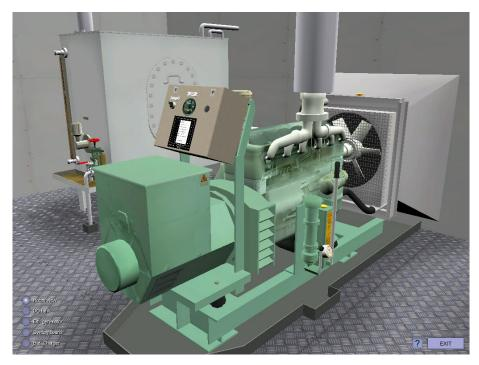
Fig.4 Emergency Power Plant simulator - Diesel engine with control panel
