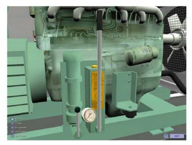
Fig.5 Emergency hydraulic starter
