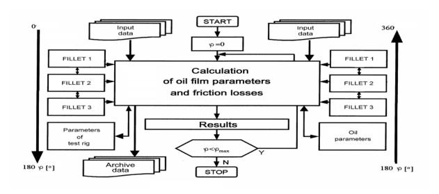
Fig. 6 Block schematic diagram of test stand mathematical model [5]
