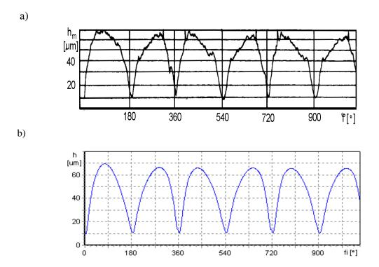
Fig. 8. Courses of oil film minimum thickness recorded on model stand (a) and for mathematical model (b)
