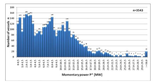
Fig. 1 Distribution of momentary power P\* [MW] calculated by Papmiel's method for vessel group tested [9]
