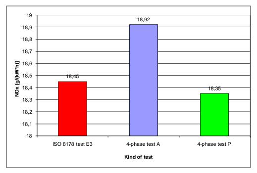
Fig.3. Comparison of NO<sub>x</sub> emission values  $[g/(kW \cdot h)]$  calculated by E3 test acc. to ISO 8170-4, 4-phase test A (required power P<sub>0</sub> determined by Admiralty's method) and 4-phase test P (required power P<sub>0</sub> determined by Papmiel's method)
