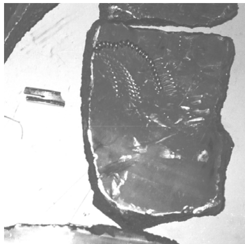
Fig.5. Spring from the piston ring pressed into the cylinder sleeve; visible black carbon deposit originated in result of incomplete combustion of cylinder oil [source:Ch.Eng. Marceli Stelmaszczuk]
