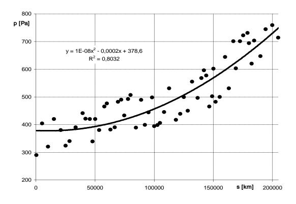
Fig. 3. Increase of exhaust gas pressure in crankcase for a cold 359 engine in the function of operational run
