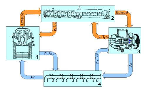
Fig. 1. The relation between particular engine's workspace areas 1 – combustion chamber, 2 – exhaust channel, 3 – turbocharger, 4 – inlet channel
