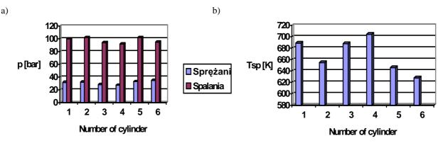
Fig. 2. Values of compression pressure and maximum combustion pressure a) and outlet temperature  $T_{sp}$  engine b) RLB66 at engine speed 188 rpm and load 76%: p - pressure
