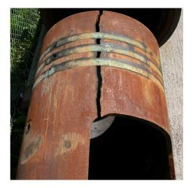
Fig 1. View of a cracked of piston skirt
