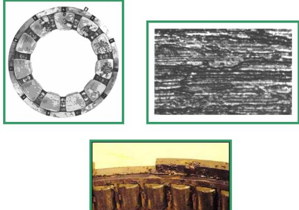
Fig. 1. The examples of bearings damage [7]
