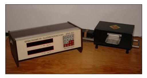
Fig.5. The fluorescence spectrometer ZBZ-93
