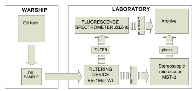
Fig. 3. The scheme of the stand for mechanical impurities in oil analysis
