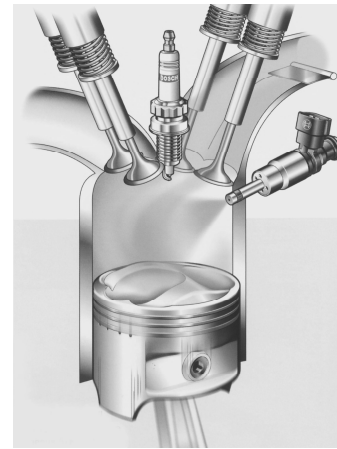
Fig. 3. The strategy of the power supply of engines with the spark-ignition and direct-injection: the homogeneous charge at big loads and rotational speeds of the engine
