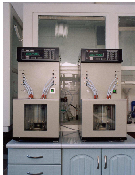
Fot. 2 Baths for kinematic viscosity measurements
