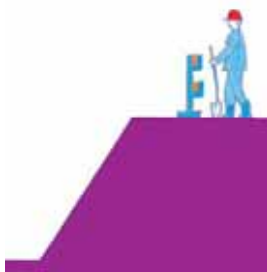
Fig. 5. A barrier used to protect against falling into an excavation
