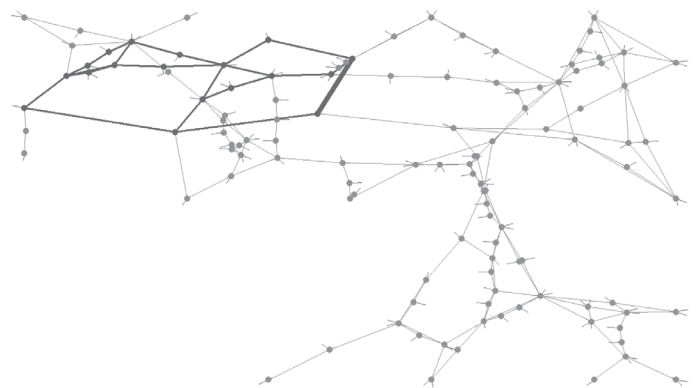
Fig. 7. Cyclical graph expansion to another area (other branches) in circulation flow development process (PST phase angle ca. 33 degrees)
