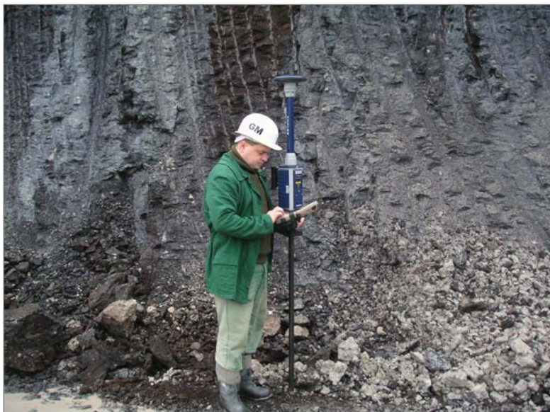
Fot. 5. Pomiar RTK z wykorzystaniem mobilnego odbiornika GPS Z-Max Phot. 5. The measurement RTK with use of mobile receiver GPS Z-Max
