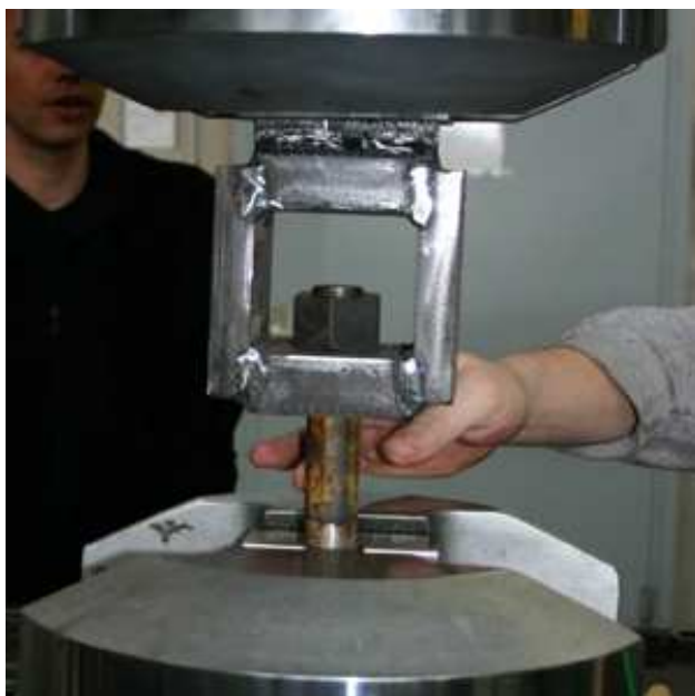
Fig. 8. Experimental set-up for the load capacity test of the screw nut.
