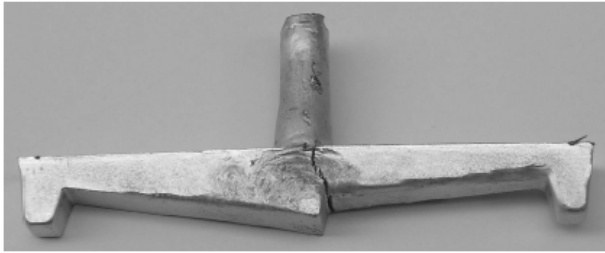
Fig. 12. Hot tearing in Al-2% Cu alloy
