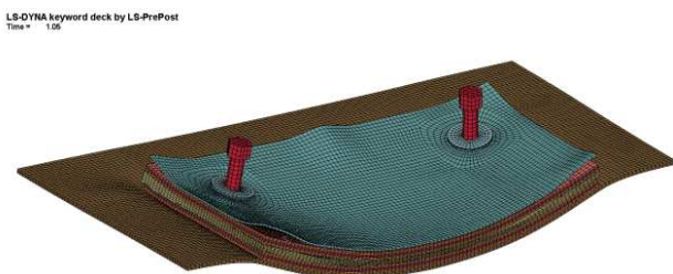
Fig. 16. The deformed protected plate – ALF panel subsystem extracted from the SPS system loaded by 6 kg TNT blast shock wave. The axonometric view on the half subsystem at t=1.05 sec corresponding to the maximum deflection of the plate
