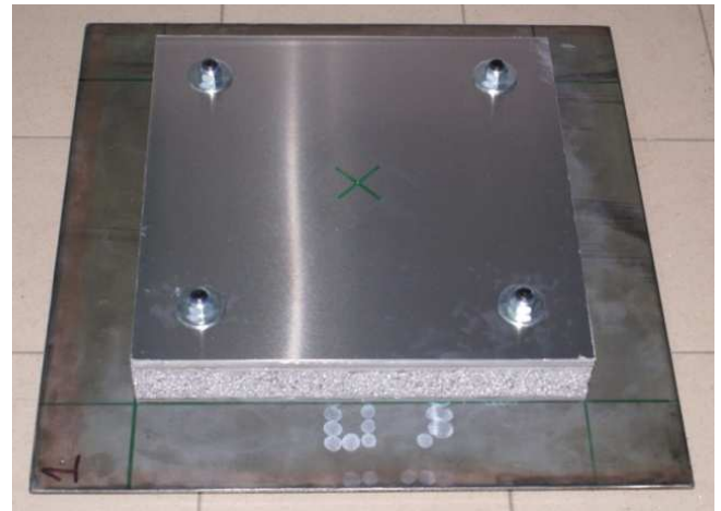
Fig. 9. Segment SP with M16 erection bolts before 6 kg g TNT blast test
