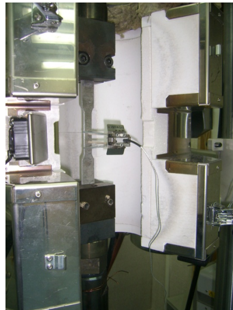
Fig. 1. The test sample and the extensometer installed inside the heating chamber (opened in the presented photo) of the Instron 8502 system
