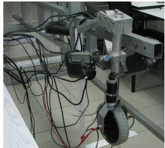
Fig. 4. Rig for testing robot leg
