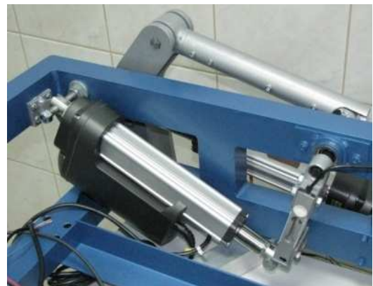
Fig. 8. Lifting drive with measuring beam
