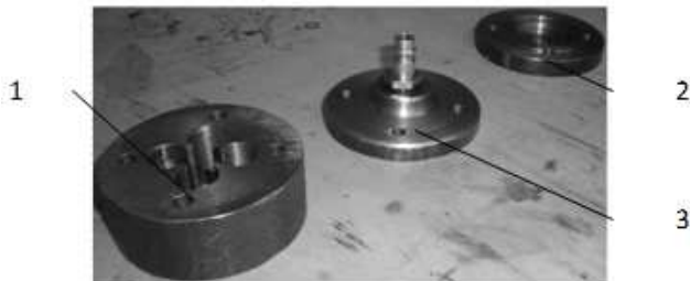
Fig. 8. Modified head of JAWA 50 engine: 1 – middle part, 2 – base, 3 - cover
