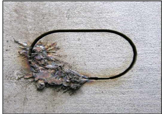
Fig. 3. A defective cutting edge
