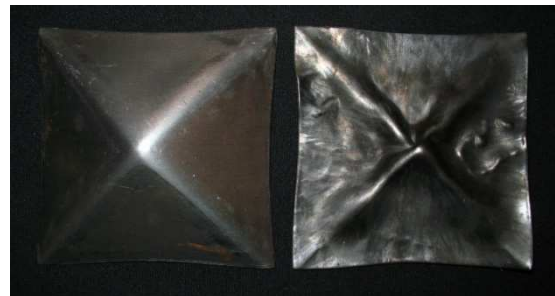
Fig. 4. Top view on deformed and undeformed pyramid
