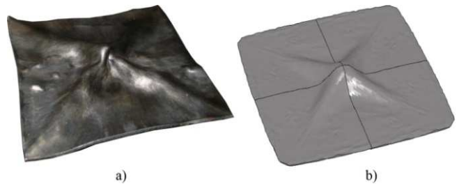
Fig. 9. Comparison of deformed pyramid from the experimental research (a) with the result obtained in full simulation of influence of pressure wave on the element (b) – top view
