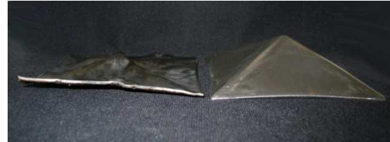
Fig. 3. Side view on undeformed and deformed pyramid
