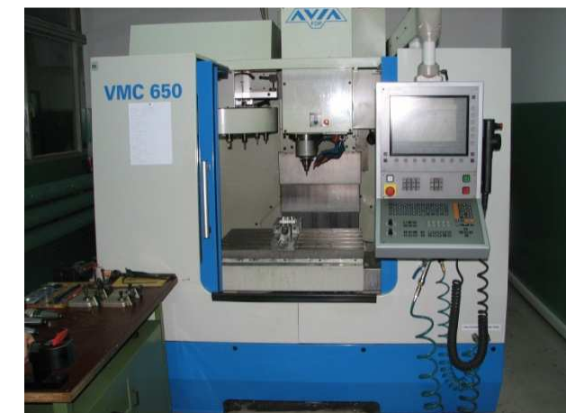
Fig. 4. Vertical machining centre used to manufacturing elements containing NURBS geometries
