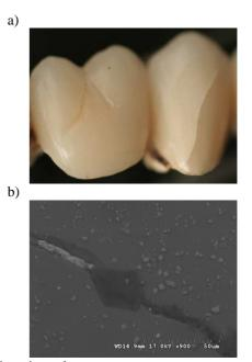
**Fig. 3.** Ceramic crack superstructure: a) macro- and b) microobservation (x900)
