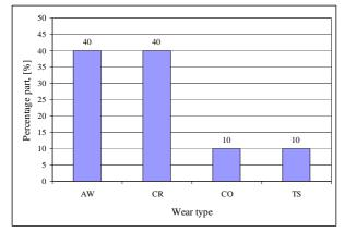
Fig. 8. Percentage damage fraction: AW – abrasive wear, CR – cracking, CO – corrosion, TS – tooth scale
