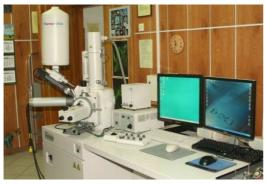
Fig. 1. Scanning electron microscope Hitachi S-3000N
