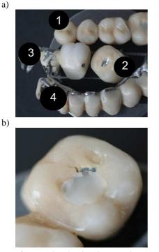
**Fig. 2.** Types of wear: 1,2 – abrasive, 3 – corrosive, 4 – microcracks; b) abrasive wear
