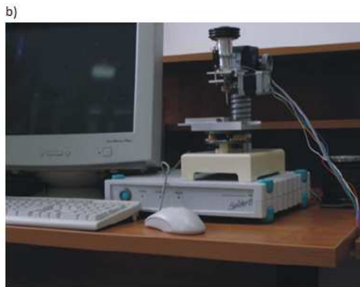
Fig. 12. The laboratory stand for dentures diagnostic (Kuchta, 2006): a) the stand's diagram, b) view of apparatus and system register
