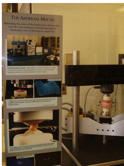
Fig.13. The stand for denture tests – artificial mouth (Studium Famulaturen&Auslandsaufenthalte)
