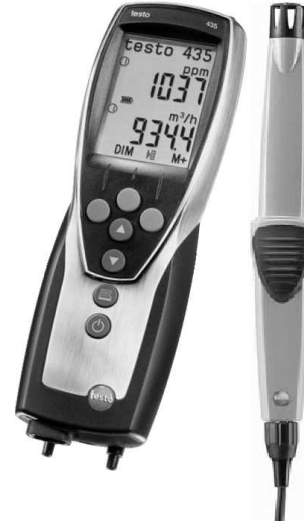
Fig. 2. Measuring instrument Testo 435 and probe to assess indoor air quality (CO 2 , humidity, temperature).
