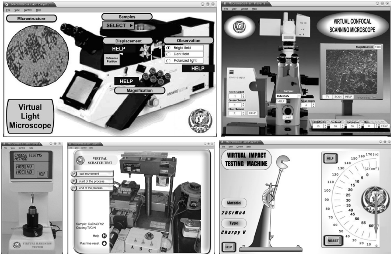
Fig. 4. Examples of virtual devices placed in the virtual laboratory a) light microscope, b) confocal microscope, c) hardness tester, d) scratch-test machine, e) impact testing machine (Dobrzański and Honysz, 2007)
