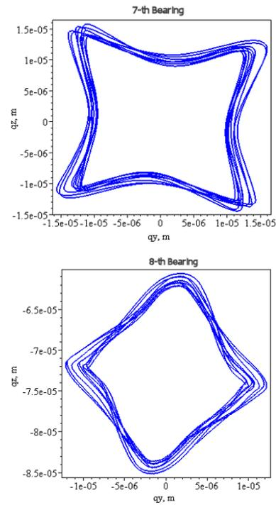
Fig. 6. Simulation results of the journals motion in the bearings at nominal rotating speed 3120rpm. a) – orbit of 7th bearing  $s_{p-pmax}=31\mu\text{m}$ , b) – orbit of 8th bearing  $s_{p-pmax}=25\mu\text{m}$
