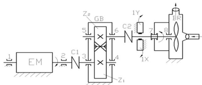
**Fig. 1.** The air blower and proximity probes location scheme: 1, 2 – journal bearings of EM; 3 - 6 – journal bearings of gearbox (GB) with transmission ratio  $u = 0.477712$ ,  $z_2 = 43$  of a driven gear and  $z_1 = 90$  of a driving gear; 7, 8 – tilting-pad journal bearings of blower rotor (BR); C1, C2 – flexible couplings; 1X, 1Y – proximity probes fixed at the 7<sup>th</sup> bearings
