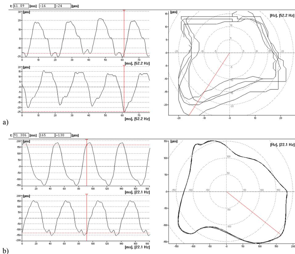
**Fig. 2.** The vibration displacements plots and orbits of blower rotor measured at bearing 7th at full loading (a):  $s_{(o-p)x} = \sim 22 \mu\text{m}$ ,  $s_{(o-p)y} = \sim 20 \mu\text{m}$  and  $s_{max} = 27 \mu\text{m}$  at 3132 rpm and at coast down, (b):  $s_{(o-p)x} = 183 \mu\text{m}$ ,  $s_{(o-p)y} = 155 \mu\text{m}$  and  $s_{max} = 210 \mu\text{m}$  at 1324rpm
