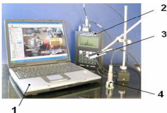
Fig. 6. The monitoring and diagnostics portable system structure (1 – Laptop with special software; 2 – data collector-analyzer; 3 – the sensor of shaft revolutions; 4 – vibration sensor)
