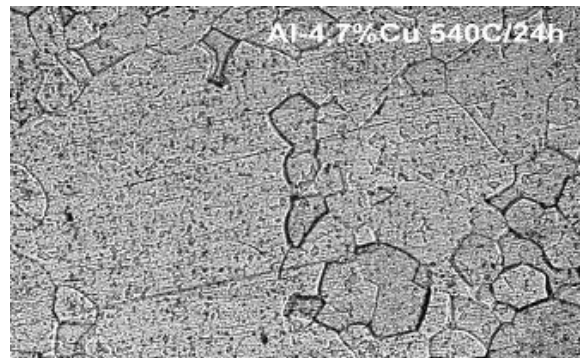
Fig. 4. Structure after annealing for 24 h at 540°C. Magnification 100 X
