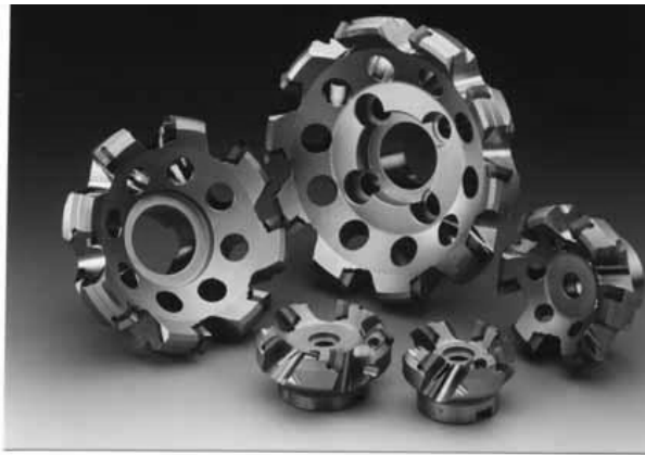
Fig. 1. Example of milling heads with different geometry [1]
