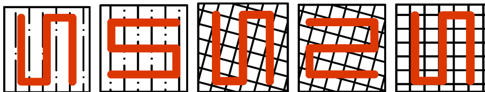
Fig. 6. Directions of the milling tool paths in relation to the fibres location in the composite
