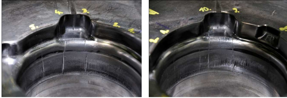
Fig. 4. Visualization of fracture repair forging tools before cutting operation
