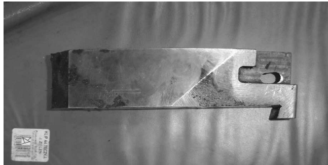
Fig. 2. Standard tool used on wheel-turning lathe
