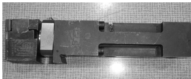
Fig. 3. Special tool with inserted force meter
