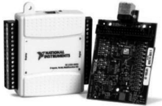
Fig. 16. A/D converter used in EB-3 (NI USB-6009; features: 14-bits resolution, sampling frequency: 48kS/s)
