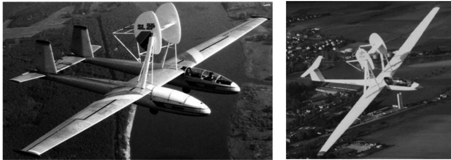
Fig. 1. Schemp-Hirth Janus glider as a fly-lab and Lithuanian fly-lab based on Blanik glider [1]
