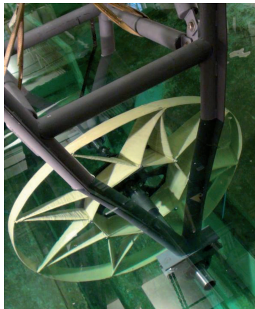
Fig. 3. CMMCT with support structure in a water towing tank
