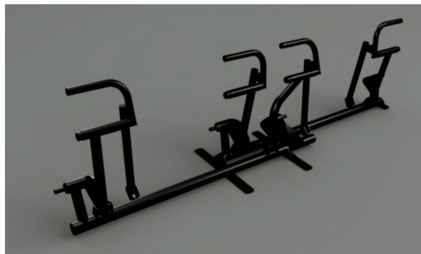
Fig. 5. Rudder pedals installation
