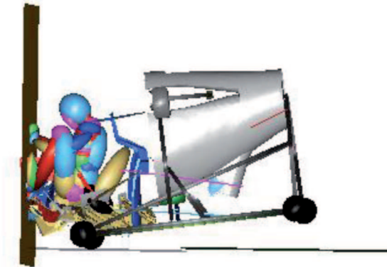
Fig. 4. Strong compression of pilot's body during the crash against the wall ( t=70 ms)
