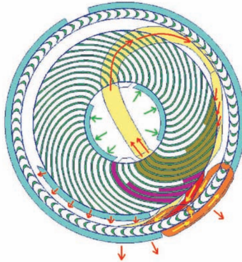
Fig. 21. Scheme of the internal flows inside the wave engine (single port set included for simplicity)
