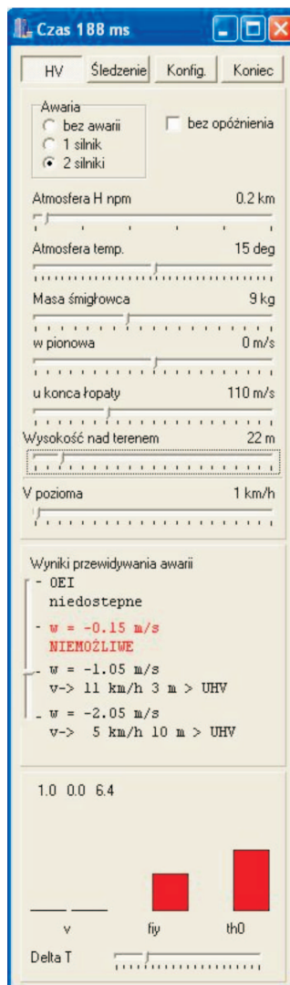
Fig. 22. Form displaying the parameters of flight and predicting the allowable maneuver in the case of engine failure. For the radio-controlled model of helicopter Benzin Trainer, autorotation soft landing with vertical speed w = -0.15 m/s will be impossible.
