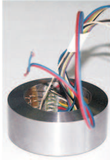
Fig. 8. The examined gasket with fixed gauges
