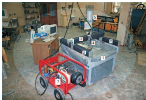
Fig. 4. General view of test stand for spatial material machining with high pressure abrasive-water jet: 1 – frame, 2 – y direction slideways, 3 – x direction slideway, 4 – abrasive-water jet working head, 5 – abrasive feed container, 6 – steering PC computer, 7 – high-pressure water pump type As500/15A
