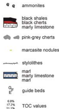
Text-fig. 3. Lithological characteristics of the Upper Hauterivian Faraoni Level and Faraoni Level equivalents from the south (Umbria Marche; Cecca et al. 1994, Baudin et al. 1994) to the north of Italy (Lessini Mountains, Dolomites; Faraoni et al. 1996, Baudin et al. 1997, Lukeneder 2010, this study). Lithology of the Puez section follows Lukeneder (2010) and includes two organic-rich black shale intervals recently discovered 50m east of the Puez 1 section. See text for details
