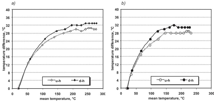
Figure 6. Distribution of temperature differences within the sections for heating with a power of 400 W: a) layer I, b) layer II (u-h – heating from above, d-h – heating from below).
