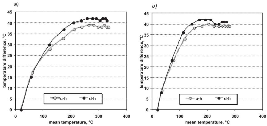
Figure 7. Distribution of temperature differences within the sections for heating with a power of 500 W: a) layer I, b) layer II (u-h – heating from above, d-h – heating from below).
