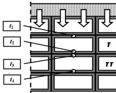
Figure 1. Schematic illustrating the arrangement of temperature measurement points within the bed. The situation shown concerns the case of heating from above.
