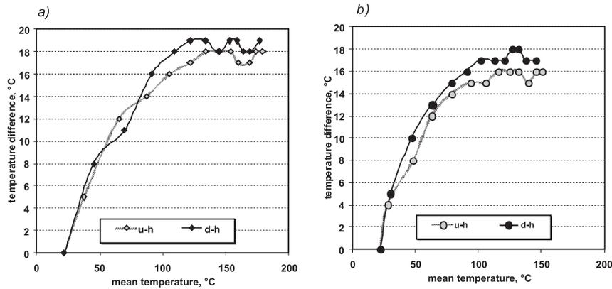
Figure 4. Distribution of temperature differences within the sections for heating with a power of 200 W: a) layer *I*, b) layer *II* (u-h – heating from above, d-h – heating from below).
