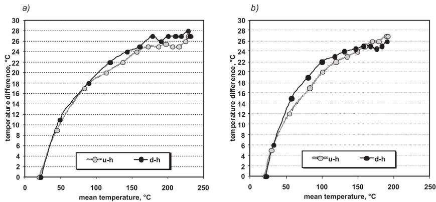
Figure 5. Distribution of temperature differences within the sections for heating with a power of 300 W: a) layer *I*, b) layer *II* (u-h – heating from above, d-h – heating from below).
