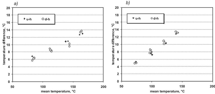
Figure 2. Distribution of temperature differences within sections as a function of mean temperature under the steady conditions of heat flow from above and from below, respectively: a) layer *I*; b) layer *II* u-h – heating from above; d-h – heating from below.
