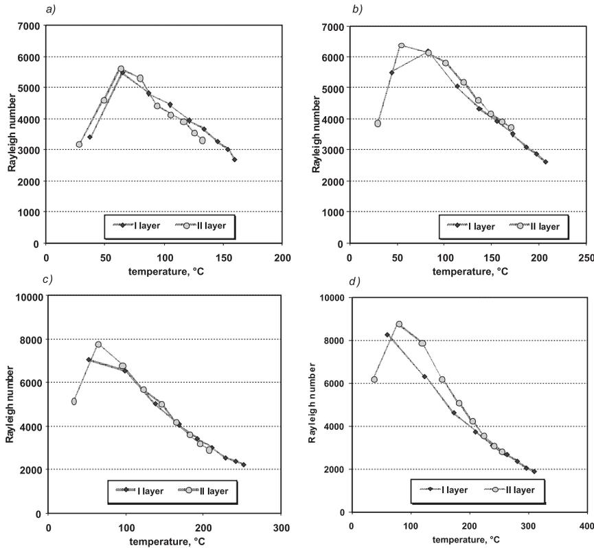
Figure 8. Developing of the Ra number value within the space of rectangular sections under unsteady heat transfer conditions: a) 200 W, b) 300 W, c) 400 W, d) 500 W.
