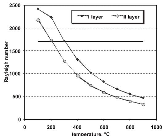
Figure 3. Results of computation of the Ra number as a function of temperature for the steady heat transfer.
