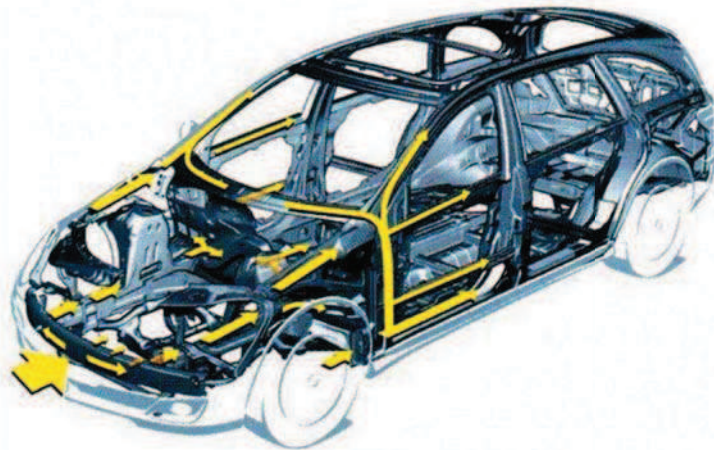
Fig. 4. Distribution of forces to specific parts of the vehicle bodywork during a frontal collision [4]
