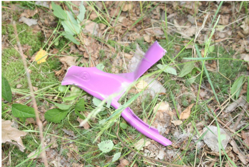
Fig. 6. Safety collar after explosion.
