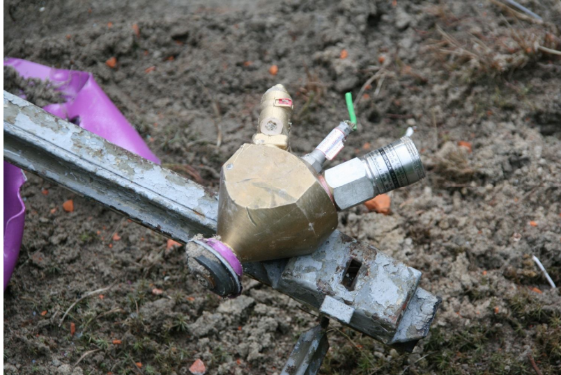
Fig. 5. Gas cylinder top with sensor outlet after explosion.
