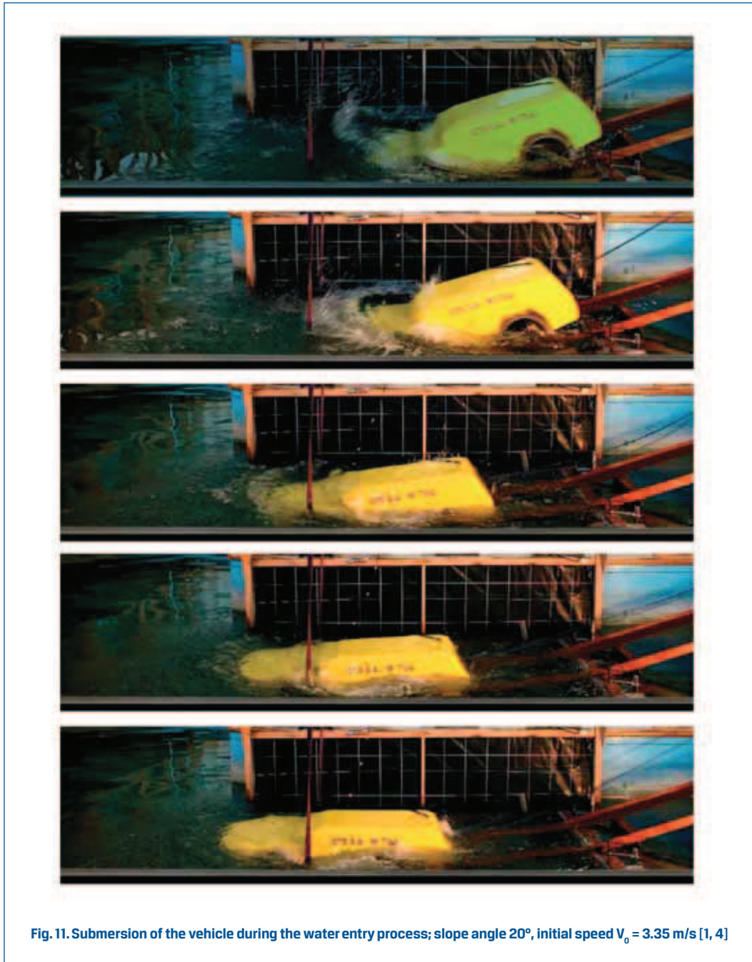
Fig. 11 shows successive stages of the water entry process as recorded during the tests; at this specific test, the slope angle and the initial vehicle speed were \alpha = 20^\circ and V_0 = 3.35 m/s, respectively.
