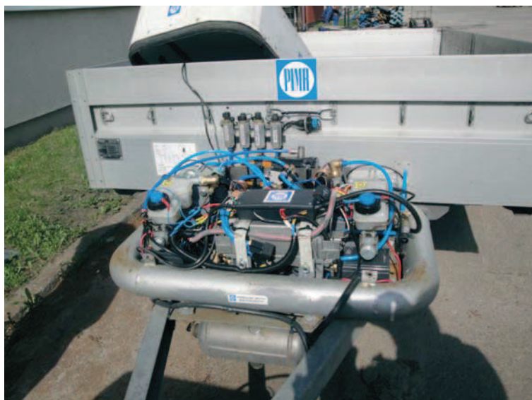
Fig. 7. The PEBS braking system in the PIMR P1 trailer (March 2010) with gel batteries within the space made of the main tank tube.
