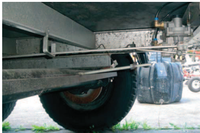
Fig. 13. LSV valve in 03 category semi-trailer.
