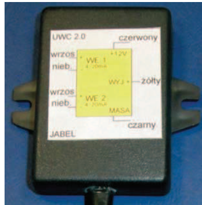
Fig. 4. View of the electrical signals comparator. The signals are being transmitted from the brake fluid pressure transducers of the towing vehicle master brake cylinder systems.
