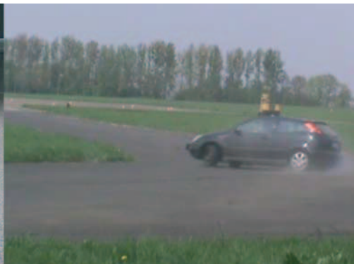
Fig.9. View of the car during drive on failed RSC tyres on rear axle (film frame).
