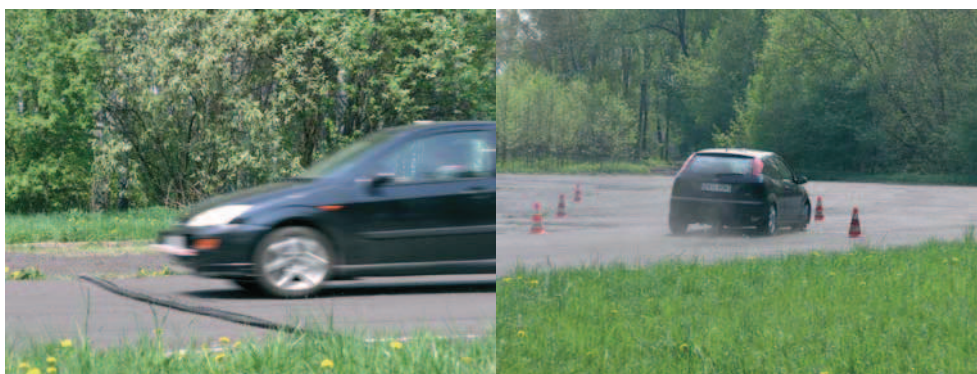
Fig. 4 and Fig. 5. The view of car driving thru spike strip and effort to driving trough the curve with punctured front wheel tyres (vehicle strongly oversteer).
