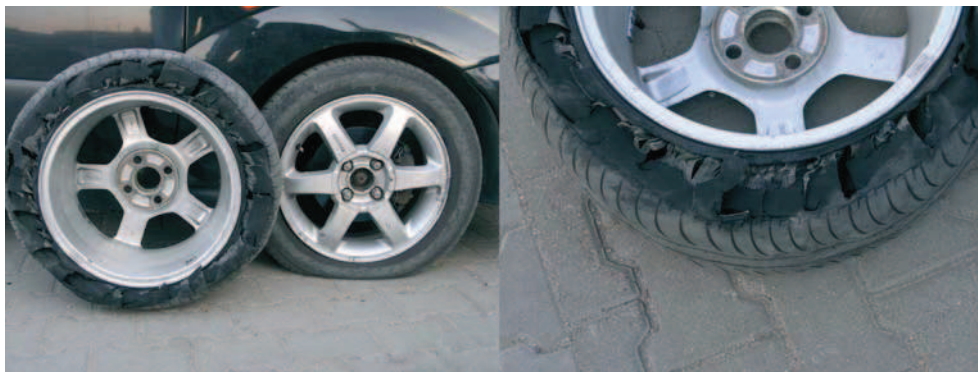
Fig 6. Comparison the visible external tyre wear of standard tyre(on left) with RSC type tyre.
