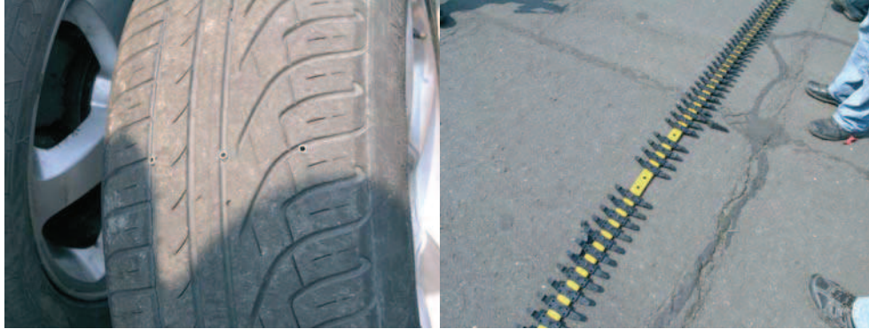
Fig.1 and. Fig 2.View the spikes drawn into the tyre and the spike strip after driving over test.
