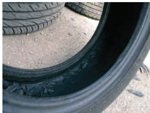
Fig.7. View the wear of internal side of RSC type tire.
