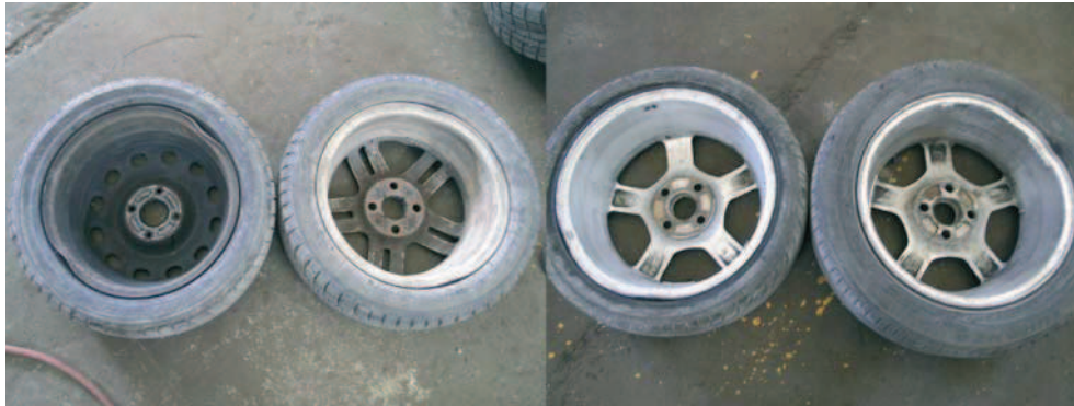
Fig.13. Comparison the defects of aluminium wheel rims with the same tyre types.
