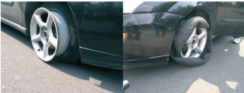
Fig. 10. and 11. View of the standard tyre damage after driving without pressure.
